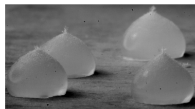
FIGURE 1 – Ice drops obtained by freezing millimeter sized water drops on a cold plate. Coupling of expansion due to solidification and capillarity effects leads to the formation of the pointy tip [1].
