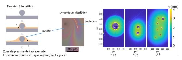
(*left*) Liquid suction around a topological defect on the glass surface. (center) White light reflection image (Newton rings) showing the accumulation of liquid around the defect and the depletion around this drop in the transient regime. (right) Thickness mapping obtained by ellipsometric microscopy around drops deposited on an oxidized silicon wafer. A nanometric film develops between the drops before they merge.
