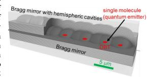
actuators. One of the mirrors has been etched using focus ion beam technology to engineer lattices of hemispheric cavities, which define a photonic lattice.
