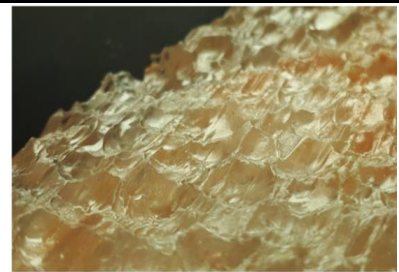
Crests formed by dissolution of salt on water, when driven by the solutal convection
