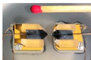
Figure 1 Left: Scanning electron micrograph of a laser-machined, ultralow-roughness mirror shape on an optical fiber. The fiber diameter is 125 \mu\text{m} . Right; Photograph of a complete FFP microcavity.
