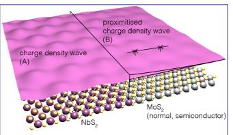
Figure: 2D transition metal dichalcogenides NbS<sub>2</sub> (type-A material) and MoS<sub>2</sub> (type-B) forming a lateral junction; by proximity effect the charge density of the former leaks out into the latter, over a certain distance before vanishing. The period and phase of the quantum wave might change upon crossing the boundary.
