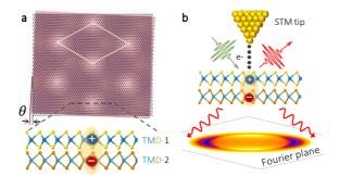
Figure: (a) Illustration of a moiré superlattice in a TMD heterostructure twisted by an adjustable angle θ. (b) STM-induced luminescence (STML) and Fourier plane imaging of excitons in a TMD heterostructure.
