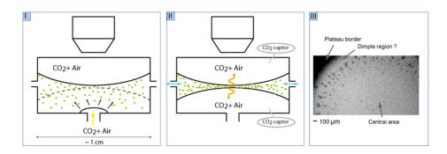
Single film experiment: a closed chamber will allow to grow a single film from a bulk suspension of microalgae (I to II). Direct vizualisation under microscope will allow to identify cell surface concentration (III) as a function of film creation parameter (flux of the incoming gas, lateral fluid flows). Once the film will be created, cell growth will be monitored as well as the CO2 consumption on each side of the film.
